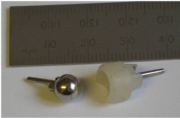
Fig. 1 The DJOA metacarpophalangeal prosthesis. The stainless steel metacarpal component is shown on the left , and the UHMWPE phalangeal component is shown on the right
