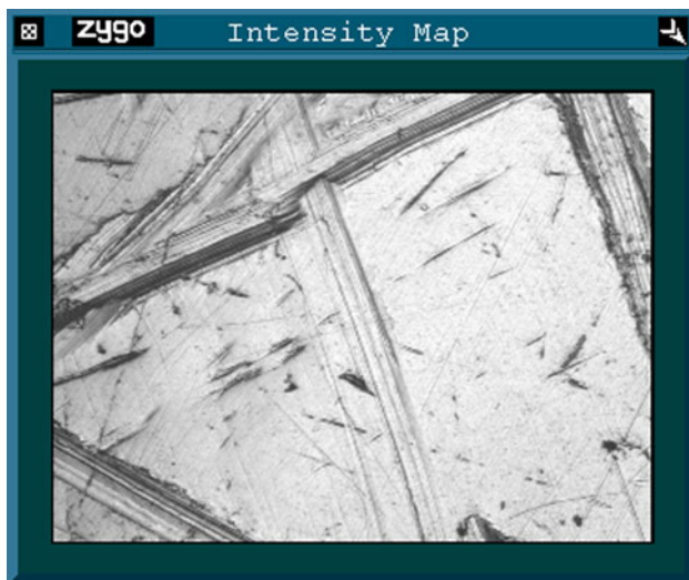
Fig. 5 ZYGO Intensity Map image of part of the surface of the metacarpal test component. Note the multi-directional nature of scratching on the surface. Scale 0.244 \times 0.183 mm
